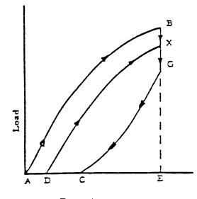
Extension FIG. 1 Determination of the Elastic Properties of Films
